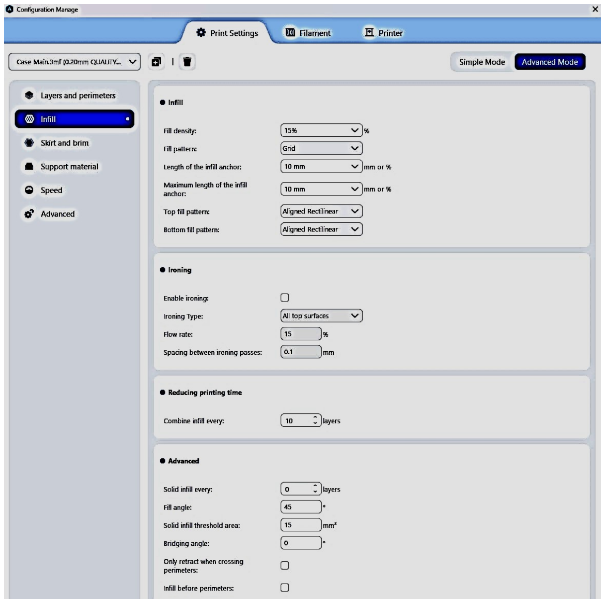
Fig. 2. Infill configuration with 15 % grid pattern and aligned rectilinear structure
