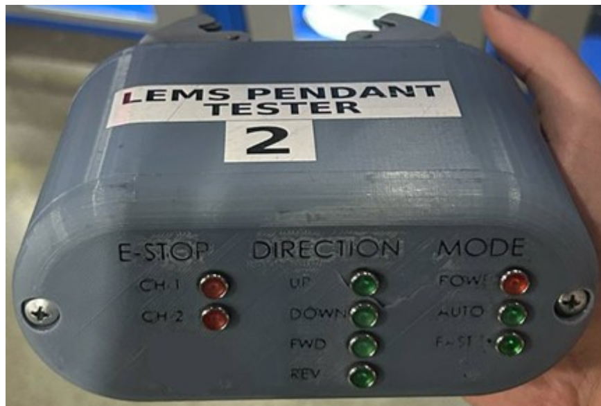
Fig. 3. Front view of the finalized 3D-printed enclosure for the industrial control unit
