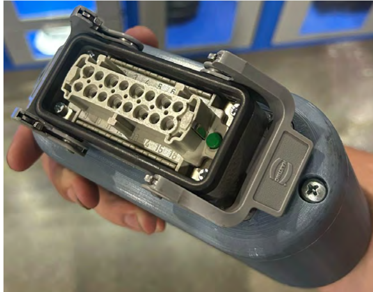
Fig. 3. Front view of the finalized 3D-printed enclosure for the industrial control unit
